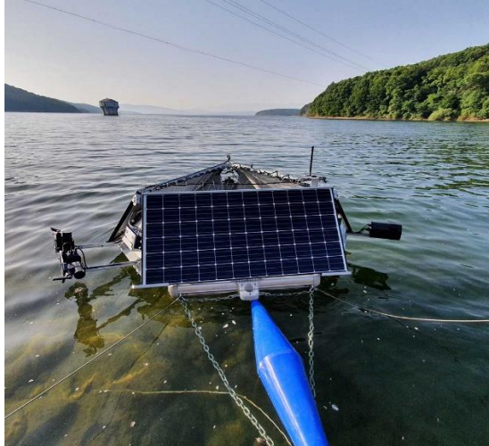
Ultrasonic Algae Control Unit (photo source: LG Sonic)
