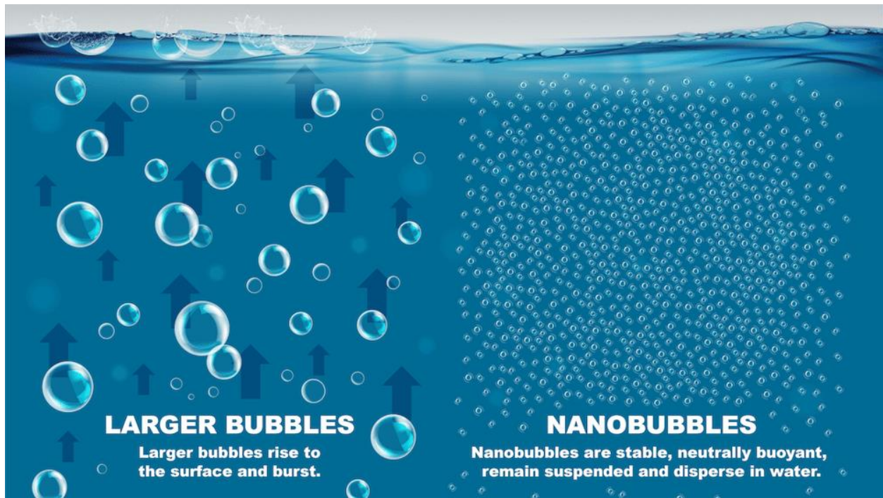
Nanobubbles compared to traditional aeration bubbles (exhibit source: Molear)
