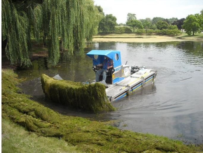
ILM's Truxor Machine Mechanically Removing Invasive Plants
