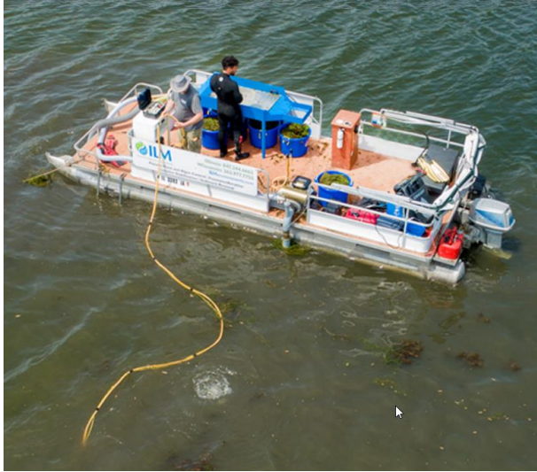
ILM's DASH Boat with Sorting Table for Wildlife Removal
