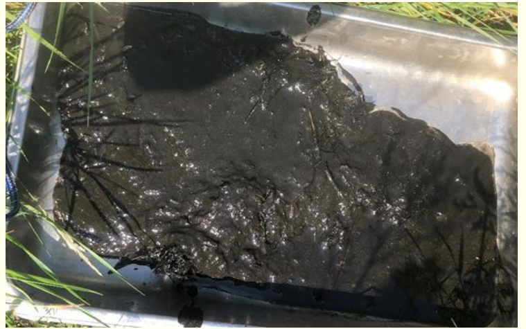
Photo #16: Kimball Channel sediment was dark brown muck. Sample collected north of Rt. 176 bridge.
