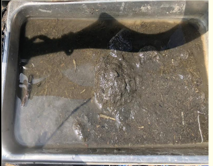
Photo #14: Berger Channel sediment consisted of peaty soil.
