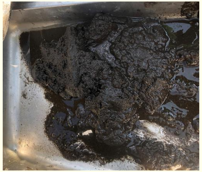
Photo #18: Washington Channel consisted of brown peaty sediment. Large snails accumulated on the Ekman dredge.
